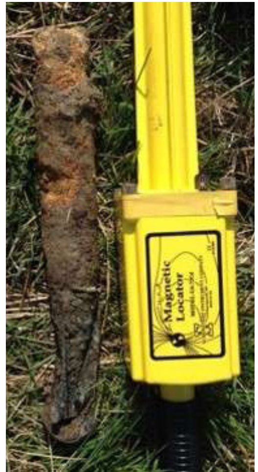
Image showing a partially expended 1kg German incendiary bomb unearthed on a development site at Avonmouth in Bristol.
