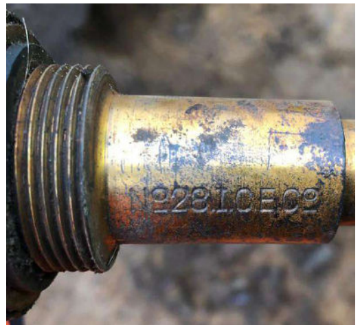
Close-up image showing a Bomb tail pistols markings after being found during ground remediation works at Full Sutton in Yorkshire.
