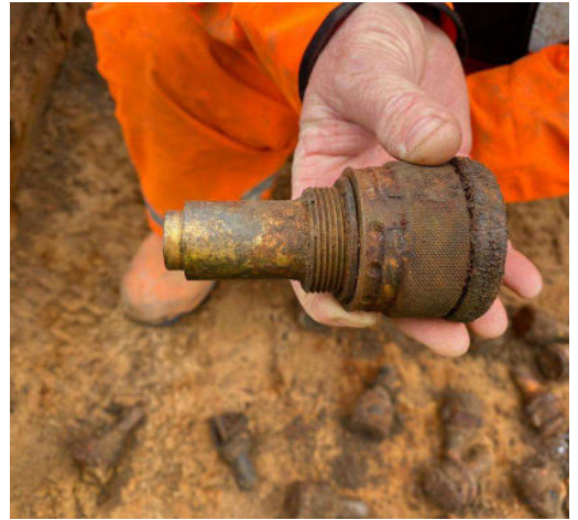
Close-up image of a Bomb tail pistol recovered during ground remediation works at Full Sutton in Yorkshire.
