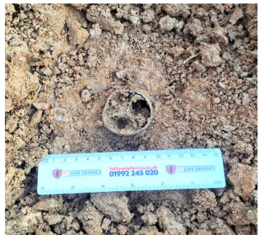
Example of one of the 1kg Incendiary Bombs discovered on-site by the Target Investigation team at East Sussex.
